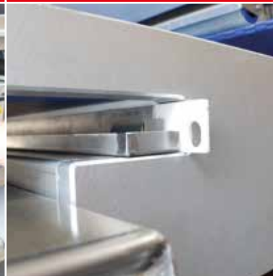
Scraper for cleaning of retracting belt
