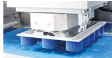
Row flexible rounding station for gentle rounding and high weight bandwidth
