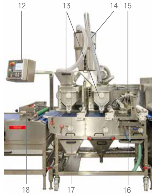
Wire belt module on a mobile frame - exchangeable with an optional conveyor belt
