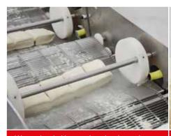
Water depth / immersion depth can be set separately for each water bath
