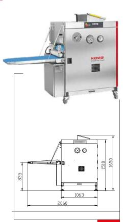
Like the Grande Rex, the Grande Rex Futura is the solution for processing high dough weights (up to 320 g). Thanks to different stamping tool sizes, it is also possible to enormously expand the range of dough piece weights.
