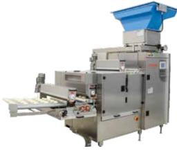
The Industrie Rex I is the classic entry-level model for high piece counts, as it can produce up to 24,000 pieces per hour. Due to the gentle dough processing with precise weight accuracy, not only the quantity but also the quality is correspondingly high.
