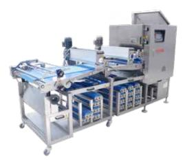
Another milestone in the weight range was set with the Rex Futura Multi. The proven Rex principle as well as the easily interchangeable dividing ledges enable the processing of an extended weight range from 12 to 245 g (rounded) or 600 g (unrounded).
