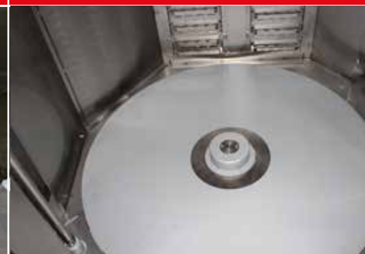
Rotating table protecting the oven floor against soiling
