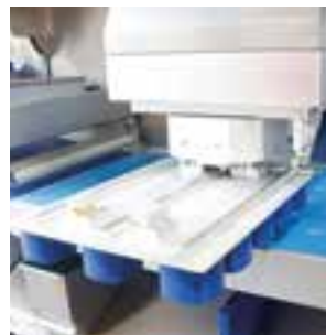
▲ Tools of rounding station can be exchanged, rounding cups are demountable
