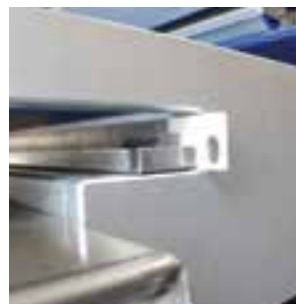
▲ Scraper for cleaning of retracting belt
