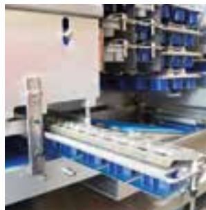
▲ Stamping station with easily changeable cutting and stamping tools
