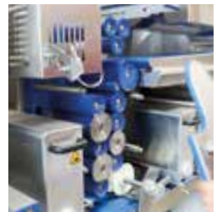
▲ Forming rollers easily extractable and adjustable for dough sheet forming
