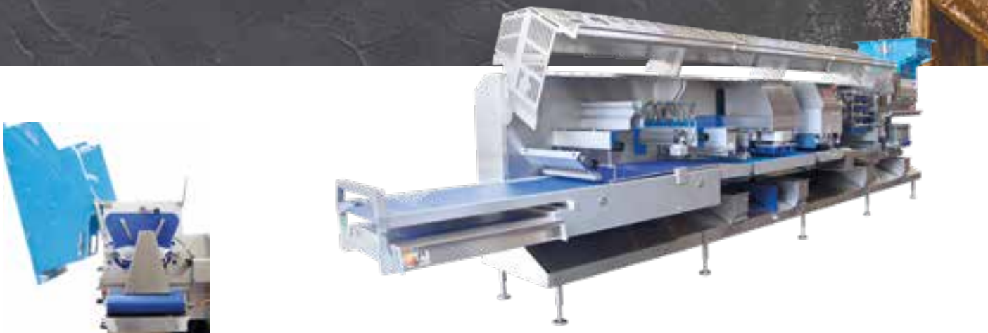
▲ Hopper can be easily folded to the side
