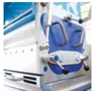
▲ Easy access to hopper rollers by removable side shield
