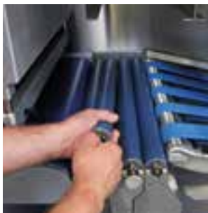
▲ Weighing cells easily extractable
