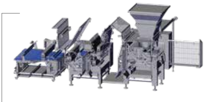
▲ Split machine: full access through the machine possible
