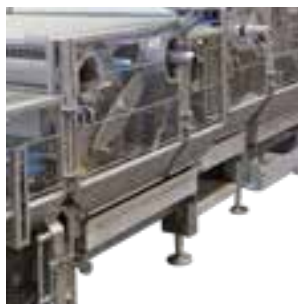
▲ Generous ground clearance prevents deposits and bevelled surfaces
