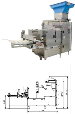
The Industrie Rex I is the classic entry-level model for high piece counts, as it can produce up to 24,000 pieces per hour. Due to the gentle dough processing with precise weight accuracy, not only the quantity but also the quality is correspondingly high.
