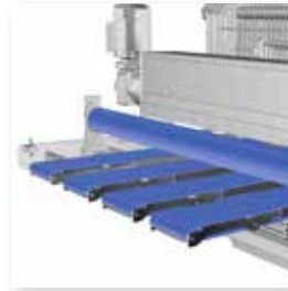
▲ Adjustable spreader straps ensure maximum flexibility and a wide range of products
